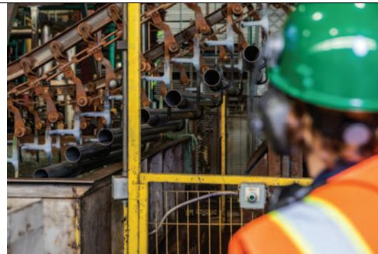
**Zinc particles adhere to the steel pipe due to electrostatic force, giving the final product a smooth, consistent and polished look. This is a unique feature of NTP's electrogalvanizing process.**
